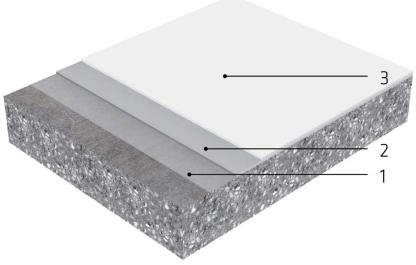
Sikalastic®-570 Top Coat is applied as UV-stable coating to enhance surface appearance as well as solar reflectivity and extend durability of Sikalastic®-612 and Sikalastic®-614 waterproofing systems.
