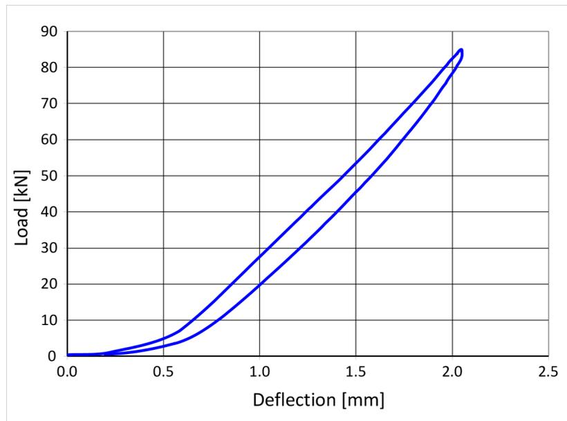
Static stiffness determined according to DIN 45673-1.
