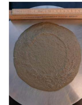
Standard mortar without SikaGrind®
