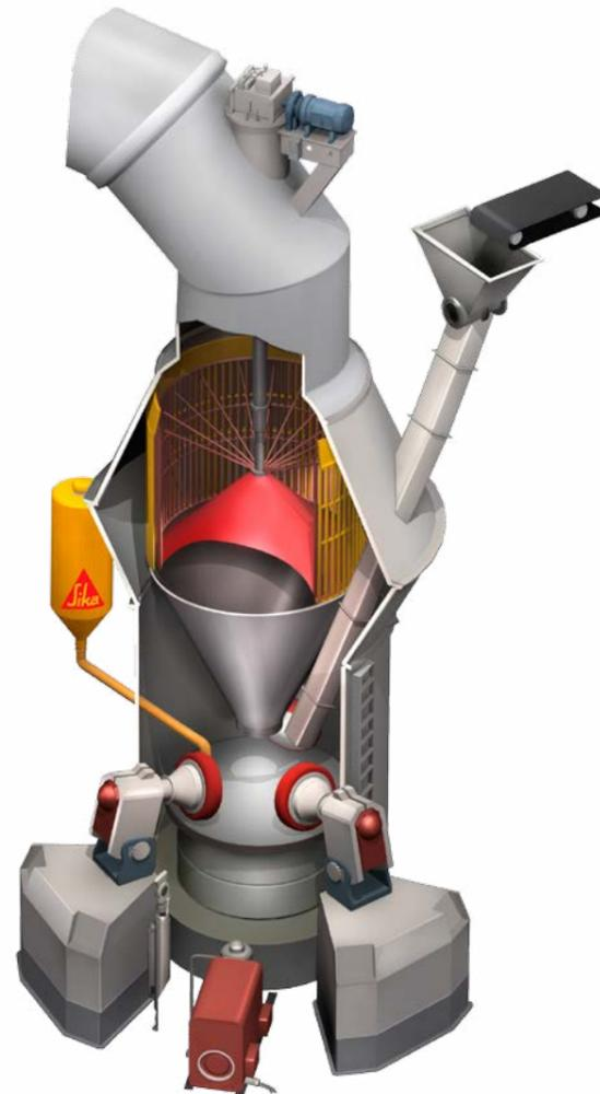
SikaGrind® is preferably sprayed onto the material bed, close to the rolls.
