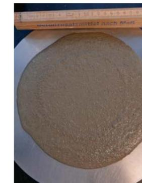
Standard mortar with SikaGrind® LS-43
