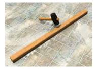
Compact well into the joints using a vibratory plate, or simply use a wood plank and hammer.
