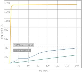
— Fire test curve — Concrete — Reinforcement steel
