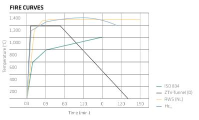
These fire exposure rating curves all simulate the temperature profile of a tunnel fire. The example of the Dutch RWS curve defines the maximum exposure which can be expected in the worst case scenario: This is defined as a fire of a road tanker truck with a load capacity of 50 m<sup>3</sup> that is 90% full of liquid hydrocarbon fuel (petrol).
