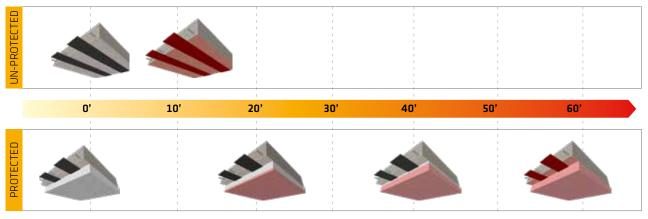
Even in the case of using protective materials applied in a considerable thickness, the expected protection will be restricted to a limited period of time (e.g. 45 – 60 minutes). A long-term protection for the CFRP strengthening (120 – 240 minutes) is not feasible unless extremely costly or complex solutions have been provided. Short-term CFRP protections do not involve a low fire resistance for the structural member.
