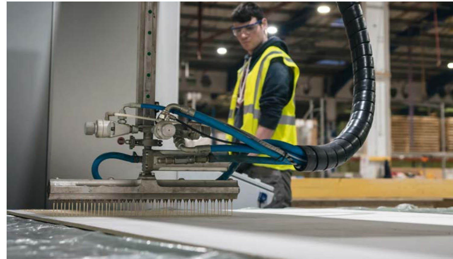
SikaForce® applied by spreader bar
