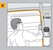
■ Using a brush apply a thin continuous coat of Sika® Primer-207 on the damaged area and let it dry for a minimum of 3 minutes.
