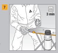
■ In case of laminated safety glass, apply a protecting layer of Sika® Primer-207 onto the edge of the glass and let it dry for a minimum of 3 minutes
