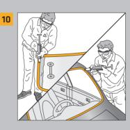
Using a triangular nozzle apply the adhesive on the glass or on the body.
