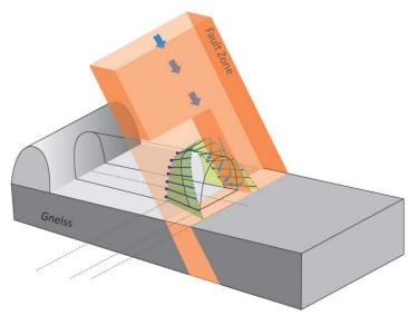
Following an assessment of the current situation, Sika's waterproofing plan was to form a sealing casing (green section on the graph) around the transverse tunnel inside the crushed zone. With the "punch-insert-punch" method, the incoming waterfront was progressively moved to the top of the front, where the final injections were performed.
