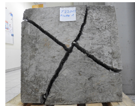
Figure 8.2.1.2: Underside view of tested square panels
