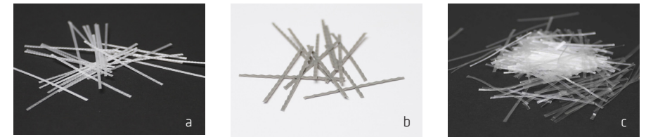
Figure 5.3.1: a) Straight embossed fibres b) Undulated fibres c) Soft flat fibres
