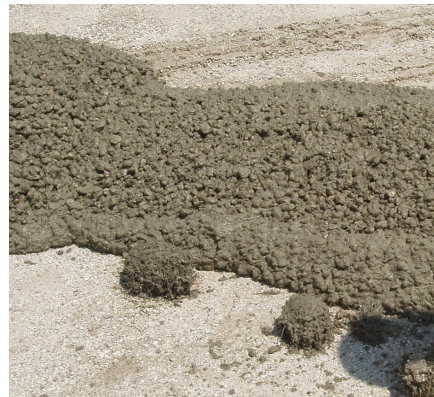
Figure 4.1.2: Fresh concrete with balling
