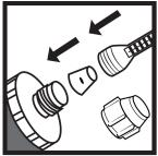
2. Fit the cartridge outlet plug into the cartridge then place injection resin mixer nozzle onto the cartridge
