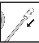
6. Fit push fit connector onto the hose. Pump gun until both resin parts are extruded as one mixed consistent colour. Do not use unmixed material. Place connector over an injection port and start the injection application.
