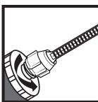
3. Slide the screwcap over the injection resin mixer nozzle and screw onto the cartridge
