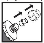
1. Unscrew the screwcap (do not throw away) and remove the plug from the cartridge outlet
