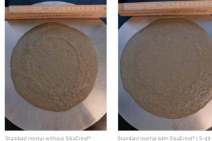
Consistence of standard mortar by flow table
