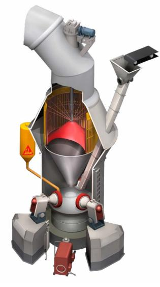
SikaGrind<sup>®</sup> is preferably sprayed onto the material bed, close to the rolls.
