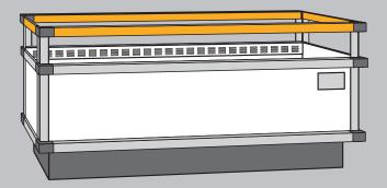
Structural bonding and sealing of organic glass on metal frame with Sikaflex®-260 N. For FDA approved applications, Sikaflex®-221 can be used. Reliable assembly of displays and small components in plastics and metals with SikaFast®-5215 NT. Body removable sealing with SikaLastomer®-710.
