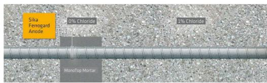
FerroGard® Patch anode simply replaces the original corrosion anode, ensuring that the steel reinforcement in the vicinity of the repair remains cathodic and protected from corrosion
