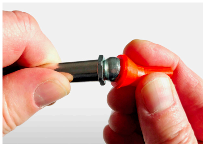
4 Apply the Flat Nozzle to the end of Application Gun
