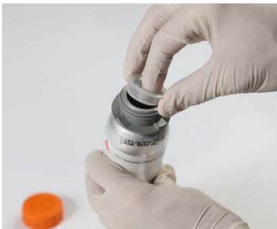
Fig. 20 Close inner cap immediately after use
