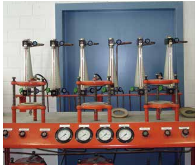
Water absorption of concrete under pressure measures the maximum water penetration in mm after a defined time with a specified pressure. (24 hours with 5 bar according EN12390-8)
