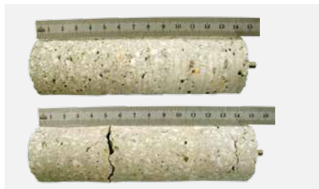
Concrete deterioration due to sulphate attack before & after the load shows a strong increase in length because of the spalling attack. First cracks have appeared in sample.
