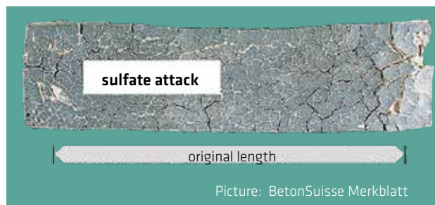
Sulfate driven attack is caused primarily by sulfates dissolved in water. By reacting with the hardened cement matrix, an increase in volume is induced which damages the structure.
