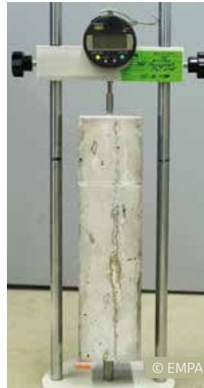
The increase in volume due to the strain resulting from ASR becomes perceptible by measurement of a change in length of test specimens. Ordinarily the specimens are stored under intensified conditions (temperature, humidity, applied load) in order to accelerate the reaction.
