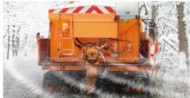
Scattered de-icing agent considerably intensifies the reaction upon freezing of water and leads to substantially greater damage in areas of concrete close to the surface.
