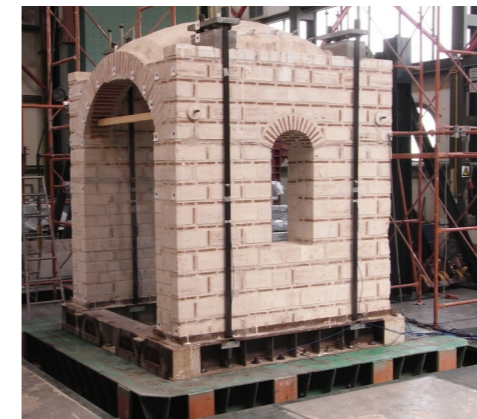
[Mouzakis Ch, et al., Seismic behavior of a rehabilitated cross vault – NIKER Project (FP7-ENV-2009-1)]
