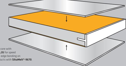
Sheet bonding on core with SikaForce®-7710 L35 for speed assembly. Manual edge bonding on off-standard products with SikaMelt®-9670.
