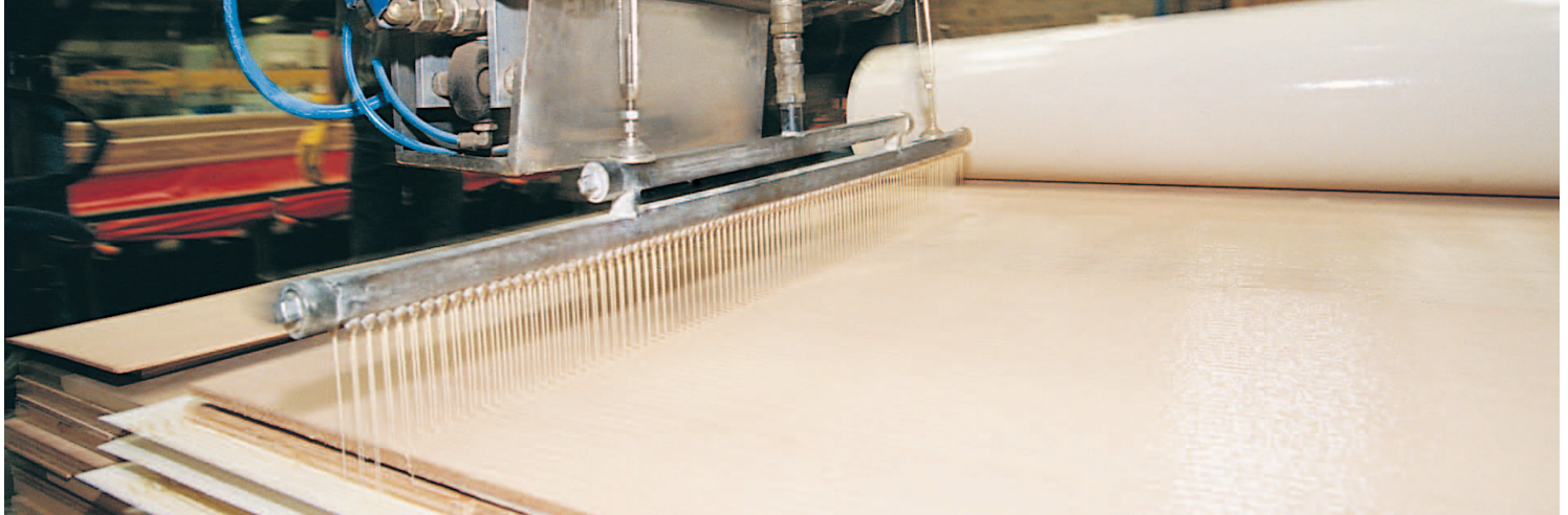
SikaForce® applied by spreader bar
