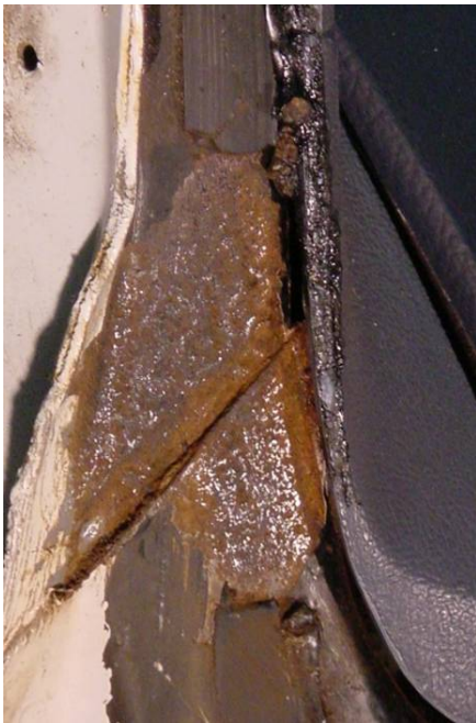
(Level 2 – 3 corrosion of pinchweld)
