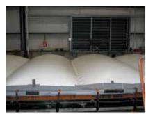
**1. WIND UPLIFT TESTING** Simulated wind uplift forces as well as testing of the pull-off strength and impact resistance for relevant fastening components to verify the wind uplift security of Sika roofing systems
