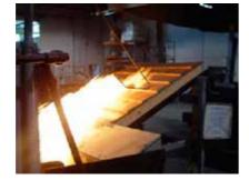
**3. EXTERNAL FIRE TESTING** Physically testing the flammability and flame propagation of the materials to verify the fire resistance of Sika roofing systems
