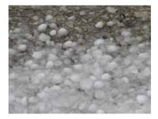
4. HAILSTONE DAMAGE TESTING Simulated hail storms are used to verify the hailstone impact resistance of the Sika roofing systems
