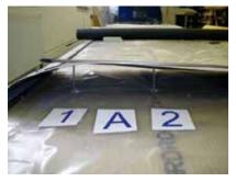
7. TEAR RESISTANCE TESTING Testing the fixings and fasteners to verify the pull-out strength and tear resistance of Sika roofing systems
