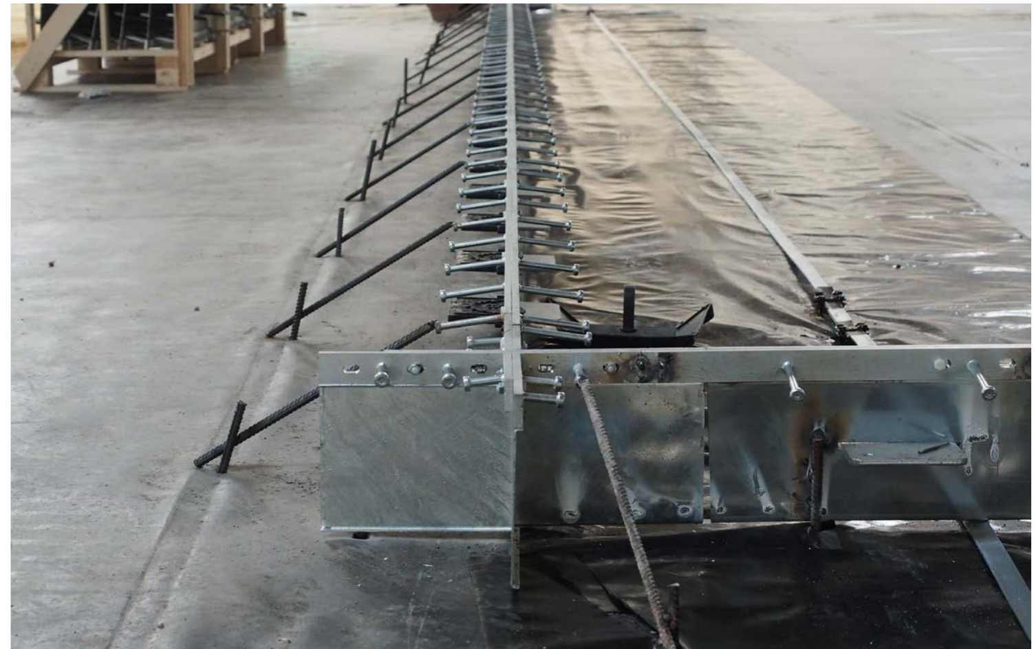
Free movement joint solution from Peikko® Group. TERAJOINT® is a prefabricated leave-in-place joint system designed to build formed free-movement joints, consisting of heavy-duty arris armor, permanent formwork and a load transfer system. It is suitable for all large-area construction methods on ground-bearing and pile-supported concrete floors.
