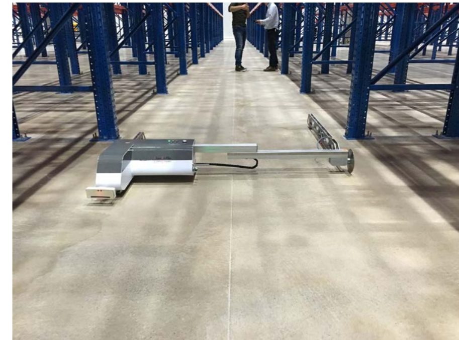
AlphaPlan FloorProfiler laser guided floor tolerance surveying robot in action.
