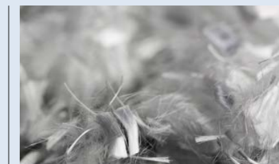
SikaFiber® (synthetic micro fiber). Typical length 6 - 12 mm. Dosage: 0.6 - 0.8 kg/m 3 .
