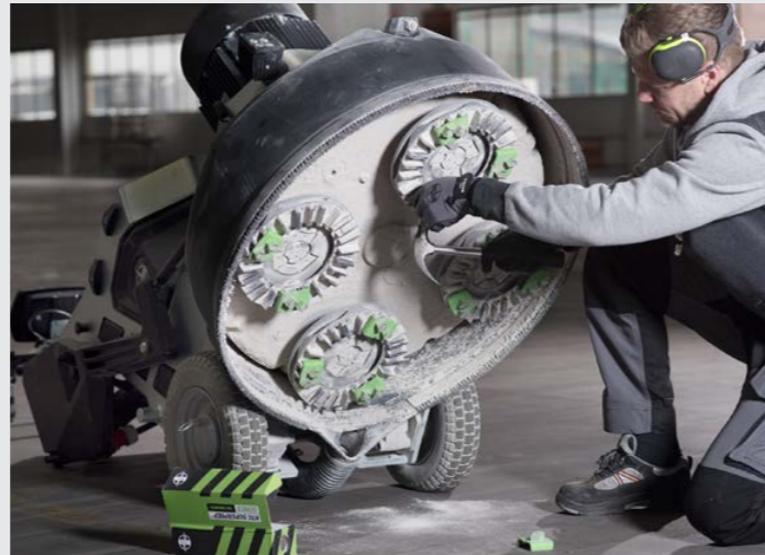
Operator changing metal bond diamond tools under an HTC DURATIQ grinding machine. The green Superprep tooling series is specifically developed for heavy preparation works.
