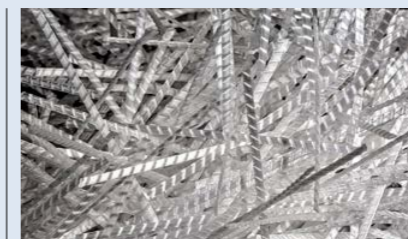
SikaFiber® Force (synthetic macro fiber). Size \Phi 1.0 mm, length 54 mm. Dosage: 3 - 8 kg/m 3 .
