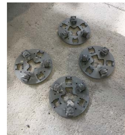
SikaScreed® HardTop-60 system requires profiled substrate. Concrete substrate was profiled accordingly by using an HTC grinding machine equipped with its special bush hammering tool "HTC Ravage".
