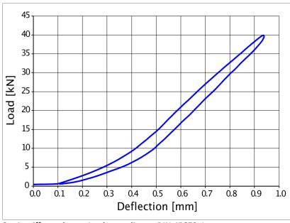
Static stiffness determined according to DIN 45673-1. Test specimen dimensions 1000 x 180 x 25 mm.
