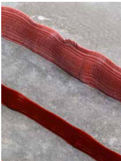
Product in normal and swelled condition after contact with water.
