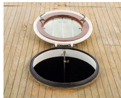
Fig. 3 A port-hatch, both bonded and sealed using Sikaflex®
