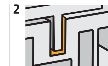
Bonding of glazing beads.
