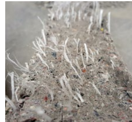
Fig. 4.6: Evenly distributed PP fibers in a broken spray test specimen.
