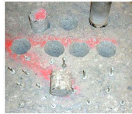
Fig. 8.6 / 8.7: Core drilling from sprayed concrete sample (left) and compressive strength measurement of a drill core (right)
