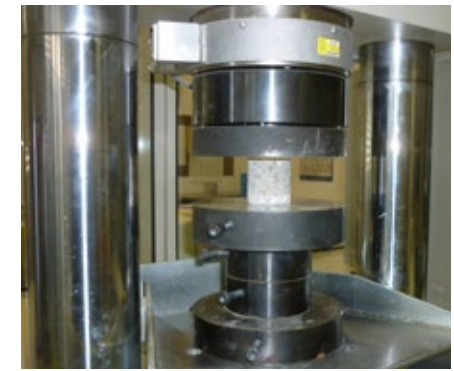
Fig. 8.6 / 8.7: Core drilling from sprayed concrete sample (left) and compressive strength measurement of a drill core (right)
