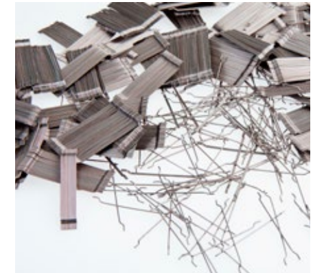
Fig. 4.7: Steel fibers for improving energy absorption of concrete specimen.
