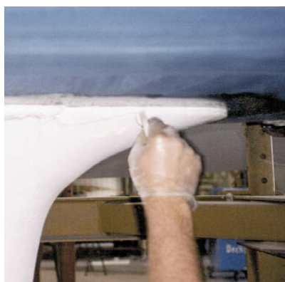
Fig. 13 The joint is tooled off and finished
