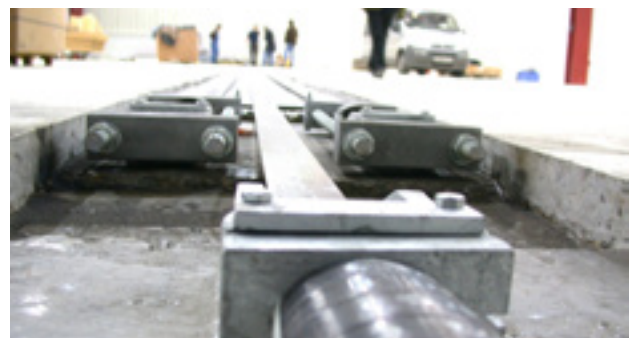
Base channel with post-tensioned CFRP plates
