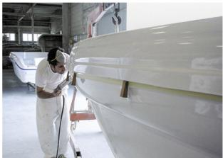
For satisfactory results the adhesive must be applied with adequate equipment such as a piston application gun. Sikaflex®-591 can be overpainted with most conventional marine paint systems.
