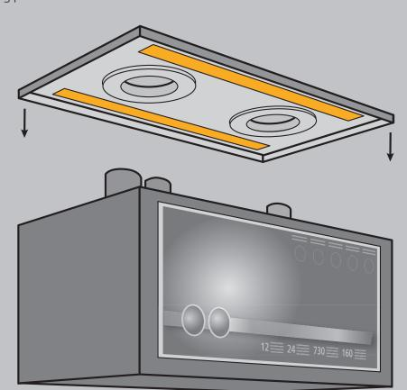
Top lid bonded and sealed with **SikaMelt®-9670**.
