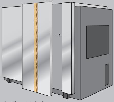
Stiffeners and metal frame structural bonding: Sikaflex®-552 AT. For faster curing, Sikaflex®-953 can be used.
