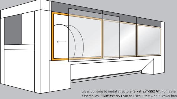
Glass bonding to metal structure: **Sikaflex®-552 AT**. For faster assemblies: **Sikaflex®-953** can be used. PMMA or PC cover bonding to metal structure: **Sikaflex®-223**. For primer-free applications, **Sikasil® AS-70** or the fast cure **Sikasil® AS-785** are advised.
