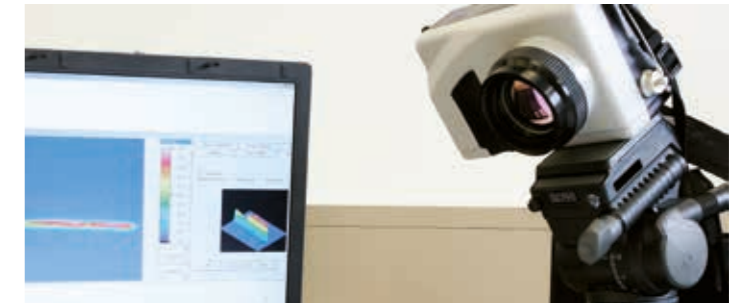
Sika System Engineering supports the optimization of the adhesive application by patented test methods. The above image shows an infrared camera measuring the adhesives heat of reaction.
