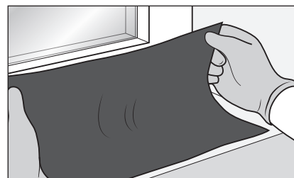
Apply SikaMembran loop-shaped and free from tension.
